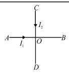
$$B = \left(B_1^2 + B_2^2\right)^{1/2} = \left[\left(\frac{\mu_0}{4\pi} \frac{2I_1}{d}\right)^2 + \left(\frac{\mu_0}{4\pi} \frac{2I_2}{d}\right)^2\right]^{1/2}$$
