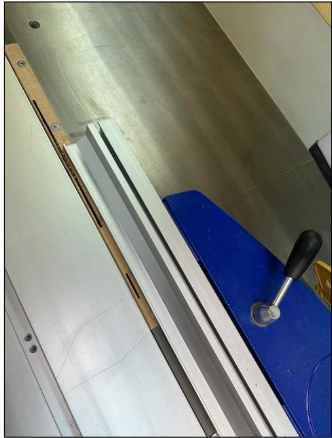
Rip fence has proper toe-out for conventional rip cuts
