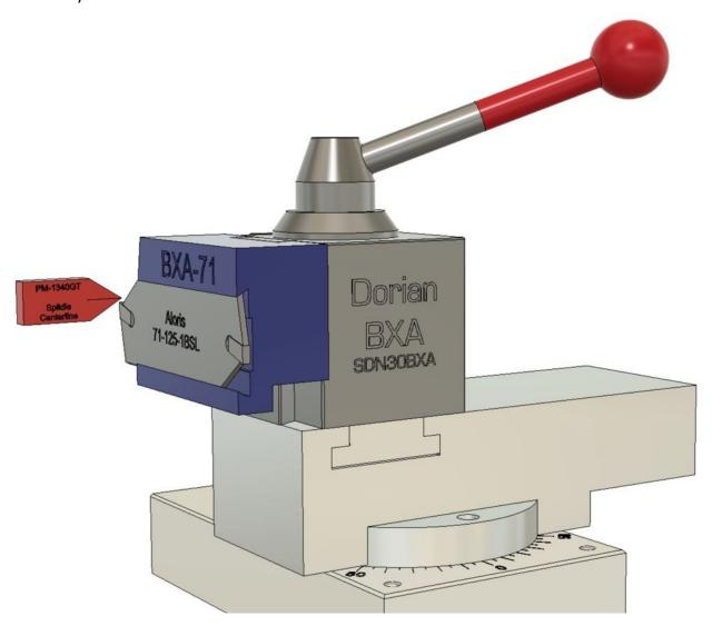
Depending on the specific brand of QCTP you own and the height of your lathe compound relative to the spindle centerline, the Aloris 77 parting blade toolholder might be a better choice. The Aloris 77 uses a different parting blade commonly referred to as a SGIH 19-3. That blade takes the same inserts as the blade that fits the Aloris 71, but the parting blade itself is half the height of the blade that fits the 71 and is thus somewhat less rigid.
