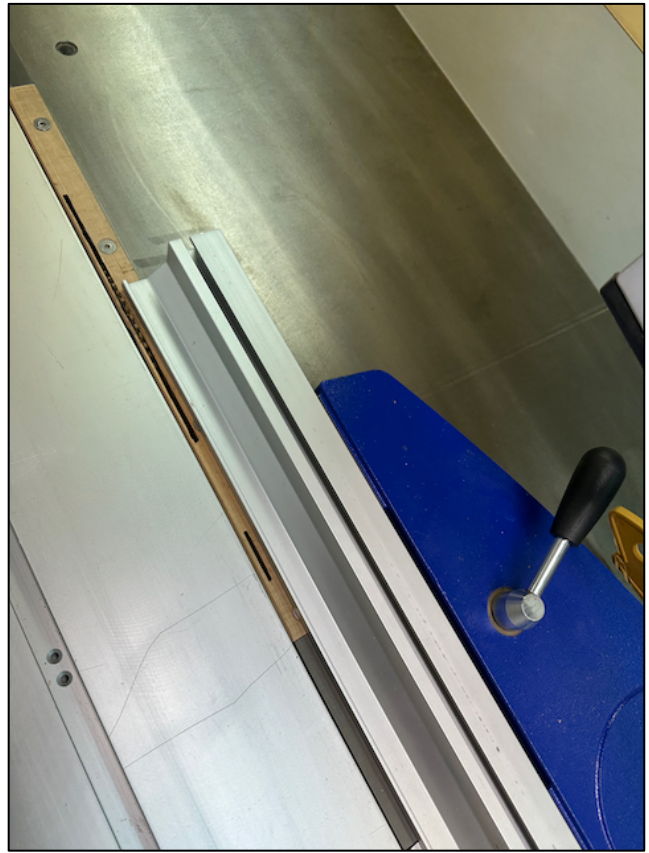
Rip fence has proper toe-out for conventional rip cuts
