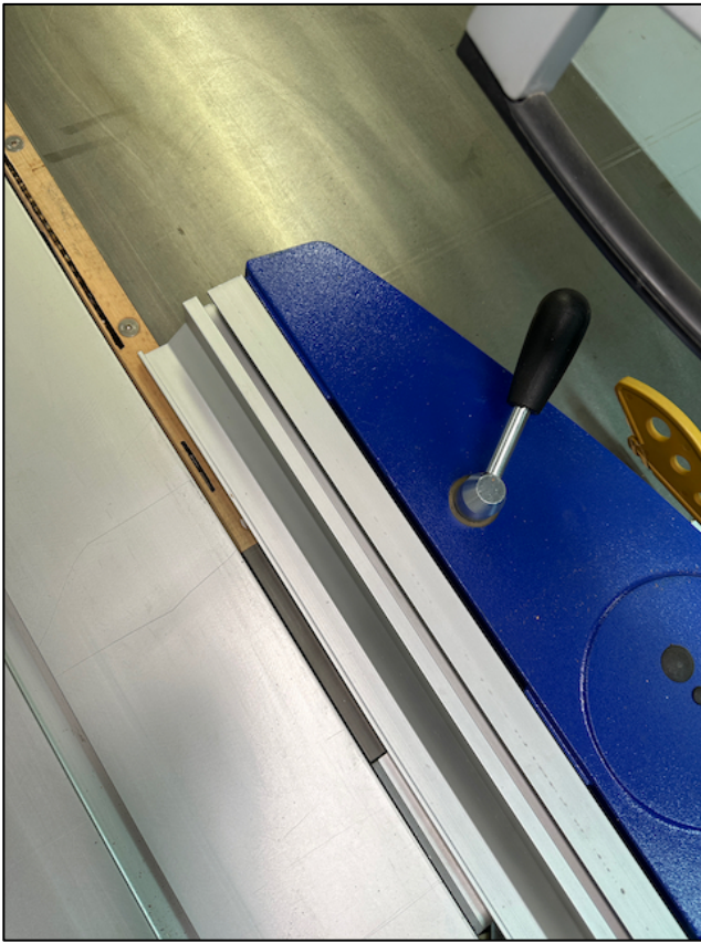
Rip fence is parallel to saw blade when retracted
