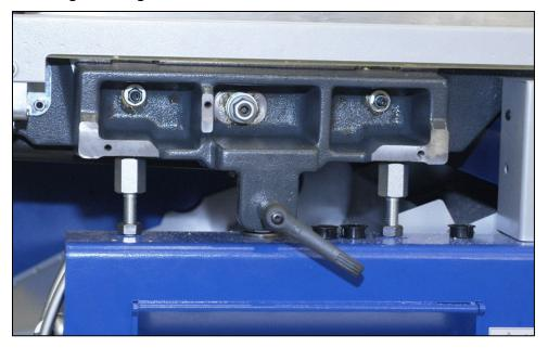
The elevation block is secured to the side of the table casting using three fasteners, which are visible above as three hex-head fasteners in the recesses of the elevation block casting. The hex-head fastener located at the center is a bolt that connects to an elevation shaft which rotates to raise and lower the table using eccentric cam lobes. The other two hex-head fasteners are nuts that help secure the elevation block to the table via threaded studs.
