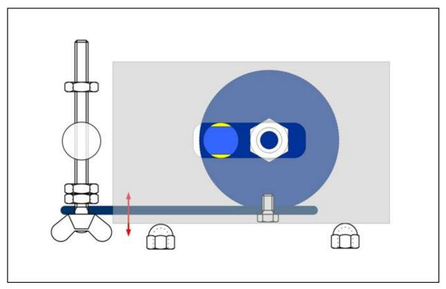
The same action occurs on the opposite side of the table – the shaft includes a matching eccentric cam element that fits into the same slot geometry on the elevation block attached to the hinge mechanism.
