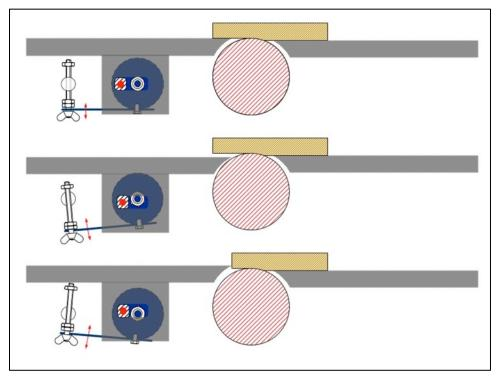
Felder moved to this new system, presumably, to simplify the manufacturing process and lower costs (the parallelogram system requires more precise manufacturing to function accurately). This cam-based "prism guide" system seems to perform well on Felder's mid-range jointer/planers up to about 16" capacity (AD731, AD741, AD941).
