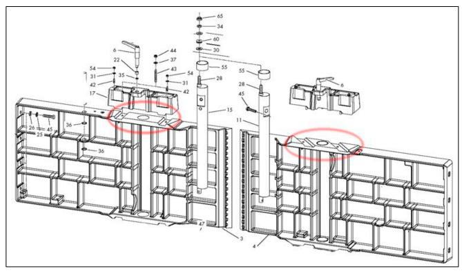
Take note of the two components circled in red. These are the prism-shaped guideways (referred to as "prism guides") that are machined into each side of the tables. The infeed table features prism guideways that are sloped, while the outfeed table has prism guideways that are oriented vertically (straight up and down).
