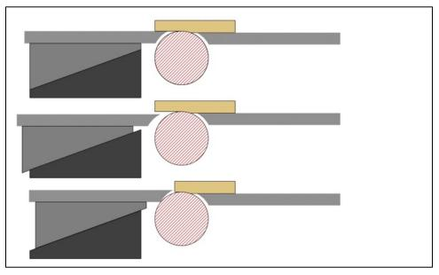
More recent designs employ a parallelogram system that elevates the tables. When properly designed and sized to the mass of the tables, this system does an excellent job of keeping the tables aligned as they move up/down. The parallelogram-type system operates as illustrated below and is used in some of the smaller Hammer machines and those made by Martin and SCMI, among others:
