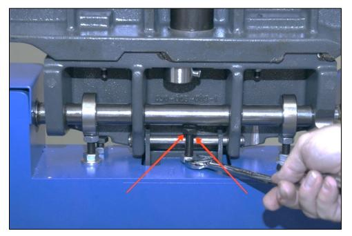
Unlike the infeed table elevation system, which moves the table up and down along an inclined plane, the outfeed table is driven straight up and down. The required vertical movement creates stiction issues between the mating prism guides making it difficult to
