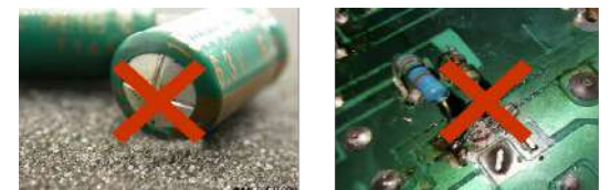
capacitor bulge and leakage
