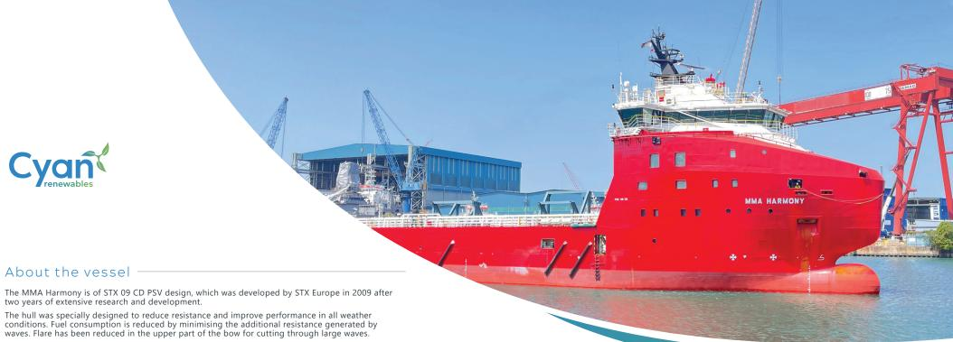
The area above the bulb is uniquely designed to reduce resistance in small or medium waves. The underwater lines are optimised for calm seas. The vessel will consume less fuel, which reduces harmful emissions to the environment.
