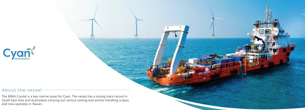
The vessel is fitted with 35T A-Frame and working class ROV as well as extensive survey equipment capable of geophysical and geotechnical operations.
