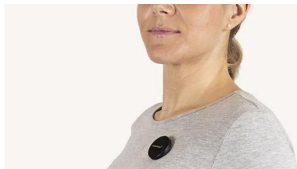
Figure 5: The Vibe Digital Sensor measures the angle user makes to a reference position, and prompts the user when the tracked angle is unergonomic [7].
