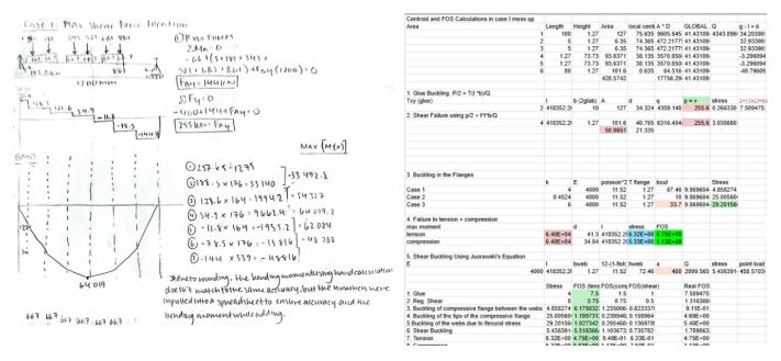
Figure 7: Using Hand Calculations, Followed by an Excel Spreadsheet for Verification. As different alterations were made, the Excel Spreadsheet Would Be Incorrect, and Needed to be Rechecked.
