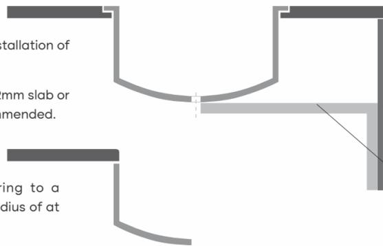
For large-size sinks, place a rod support structure under the sink so the weight is on the rods and not the countertop.
