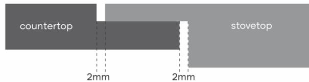
The minimum distance between the countertop and a stovetop must be 2mm.
