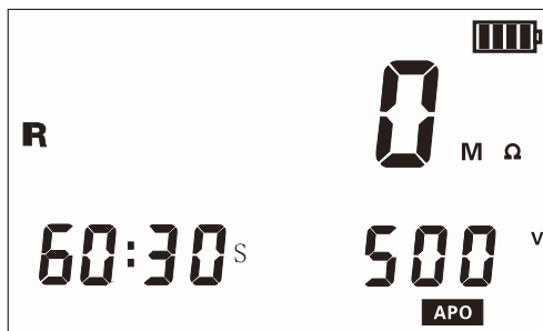
Figure 9-2 Absorption ratio mode 30 seconds mode
