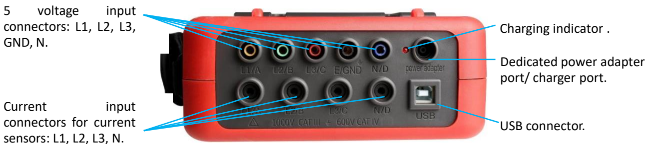
Figure 3-3: Connectors on the top of device
