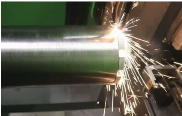
Prime Diamond Core Bit Laser Welding in progress
