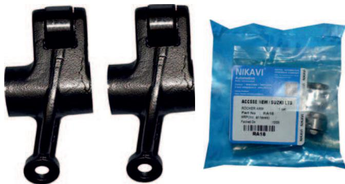
A rocker arm is an oscillating lever that conveys radial movement from the cam lobe into linear movement at the poppet valve to open it. One end is raised and lowered by a rotating lobe of the camshaft while the other end acts on the valve stem.
