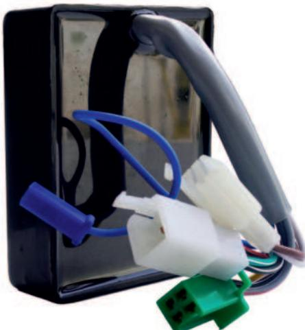
The capacitor discharge ignition system has a short transient response, a fast voltage rise (between 3 to 10 kV/  $\mu$ s) compared to inductive systems (300 to 500 V/  $\mu$ s), and a shorter spark duration (about 50-80  $\mu$ s). The fast voltage rising makes CDI systems unaffected to shunt resistance.
