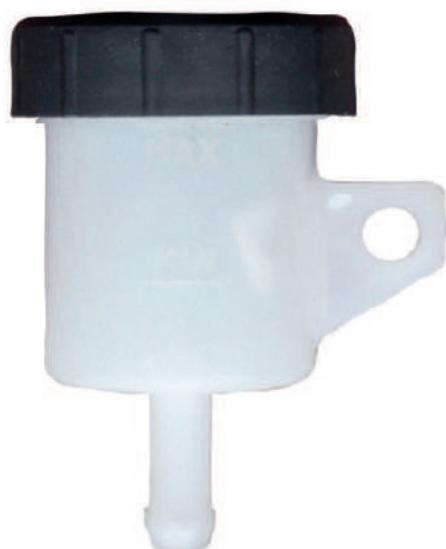
Those are the fluid reservoirs for the hydraulic front brake and depending on the bike the hydraulic clutch as well. Keep them topped up to full and flush the fluid out for fresh fluid every 5–8 years.
