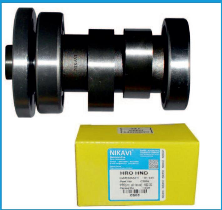
In internal combustion engines with pistones, the camshaft is used to operate poppet valves. It consists of a cylindrical rod running the length of the cylinder bank with a number of lobes, one for each valve. The cam lobes force the valves open by pressing on the valve, or on some intermediate mechanism, as they rotate.
