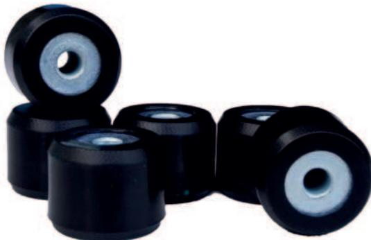
Roller weights are all set up between the variator and the ramp plate. Starting from the spinning of the scooter engine, the variator set spins. Once you open the throttle, the roller weights inside are going outward because of the centrifugal force.
