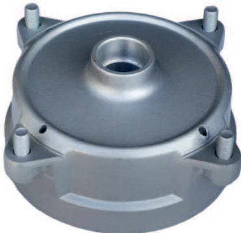
Drum brakes allow simple incorporation of a parking brake. Drum brakes are also occasionally fitted as the parking (and emergency) brake even when the rear wheels use disc brakes as the main brakes. Many rear disc braking systems use a parking brake in which the piston in the caliper is actuated by a cam or screw.
