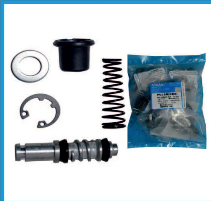
Master Cylinder As piston(s) move along the bore of the master cylinder , this movement is transferred through the hydraulic fluid , to result in a movement of the slave cylinder(s) . The hydraulic pressure created by moving a piston ( inside the bore of the master cylinder) toward the slave cylinder(s) compresses the fluid evenly.
