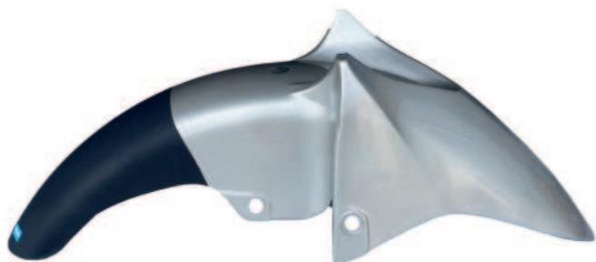
A mudguard, fender or wing is a part covering the wheels of a vehicle to stop it from throwing off mud, water or objects from the road. It protects people and property from dirtiness, dampness, and damage.
