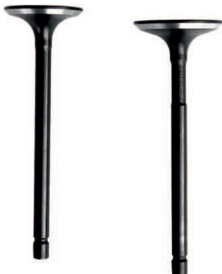
Engine valves are mechanical components used in internal combustion engines to allow or restrict the flow of fluid or gas to and from the combustion chambers or cylinders during engine operation
