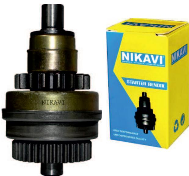
A Bendix drive is a type of engagement mechanism used in starter motors of internal combustion engines. The device allows the pinion gear of the starter motor to engage or disengage the flywheel of the engine automatically when the starter is powered or when the engine fires, respectively.
