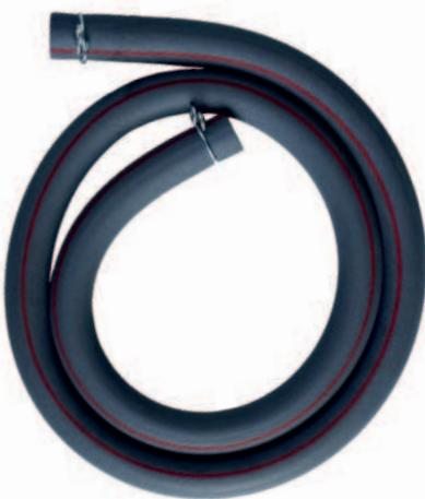
Most vehicles have rubber fuel hoses connecting the fuel pipes on the chassis to the fuel pump or carburetor on the engine. Rubber hoses are flexible and can be cut to length as required, but they have a tendency to perish over time and can rub through if not properly secured.
