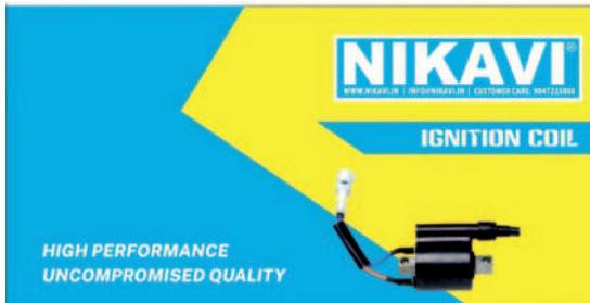
The ignition coil on a motorcycle serves to step up the relatively low battery voltage to the high voltage needed to fire a spark plug. Coils are generally a sealed, water-tight component. As such, they are generally not a repairable item. Routine checks on a coil are not necessary.
