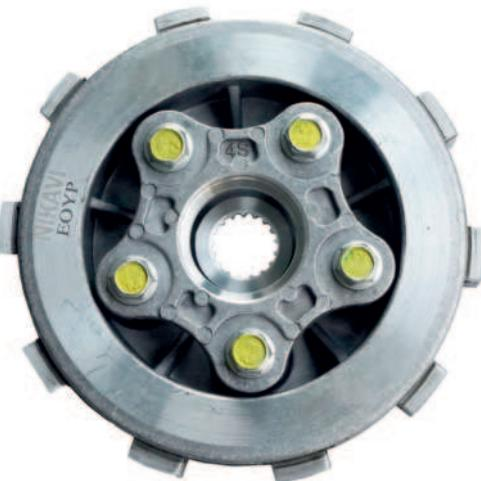
An inner clutch assembly consists of a clutch housing, a clutch hub, a clutch centre, clutch plates (friction plates and steel plates), a clutch lifter, clutch springs and bolts. The clutch assembly disengages/engages with the crankshaft of the engine to transmit power to the input shaft of the gearbox.
