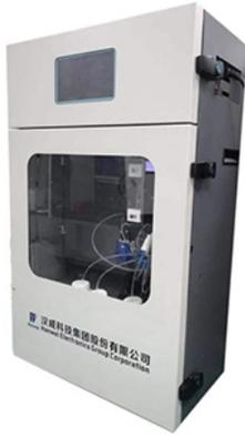
Measurement principle: COD Potassium Dichromate Method, Salicylic Acid Spectrophotometry , Total Phosphorus and Total Nitrogen Spectrophotometry
