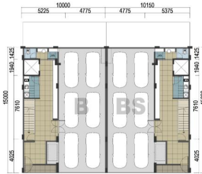
Denah Semi Basement
