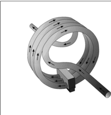
Fig. 2-107: Bent Single Pipe Design
