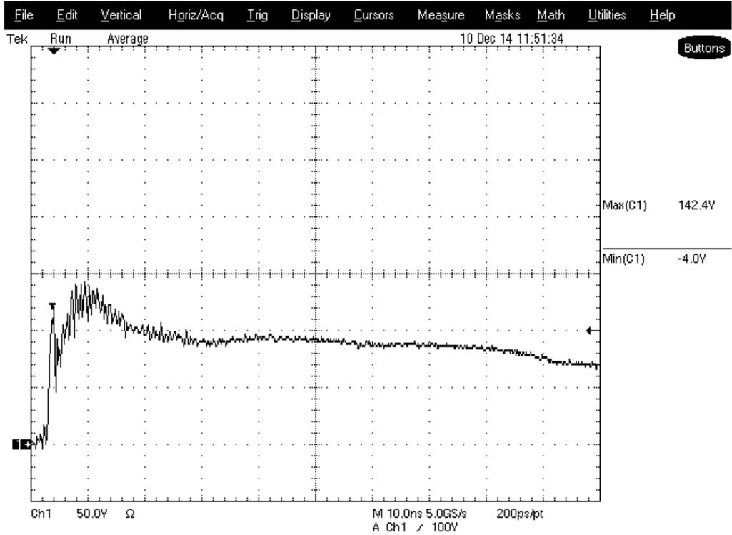
Figure 12. IEC 61000-4-2 Test Signal, +8 kV, 2 TVS Diodes and C1 = 2 nF, C2 = 33 pF, R = 15  $\Omega$  Mounted
