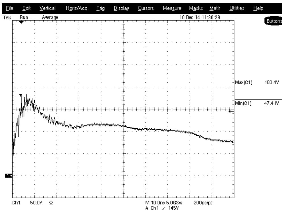
Figure 11. IEC 61000-4-2 Test Signal, +8 kV, TVS Diode and C1 = 2 nF, C2 = 33 pF, R = 15 Ω Mounted
