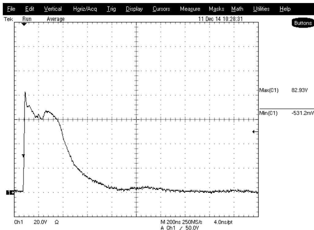
Figure 14. IEC 61000-4-2 Test Signal, +2 kV, 2 TVS Diodes and C1 = 2 nF, R = 15 Ω Mounted, Extended Time Scale
