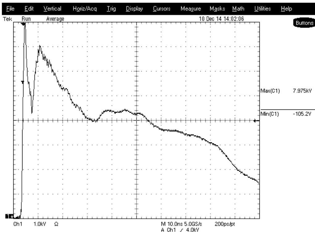
**Figure 6. IEC 61000-4-2 Test Signal, +8 kV, without Protection**
