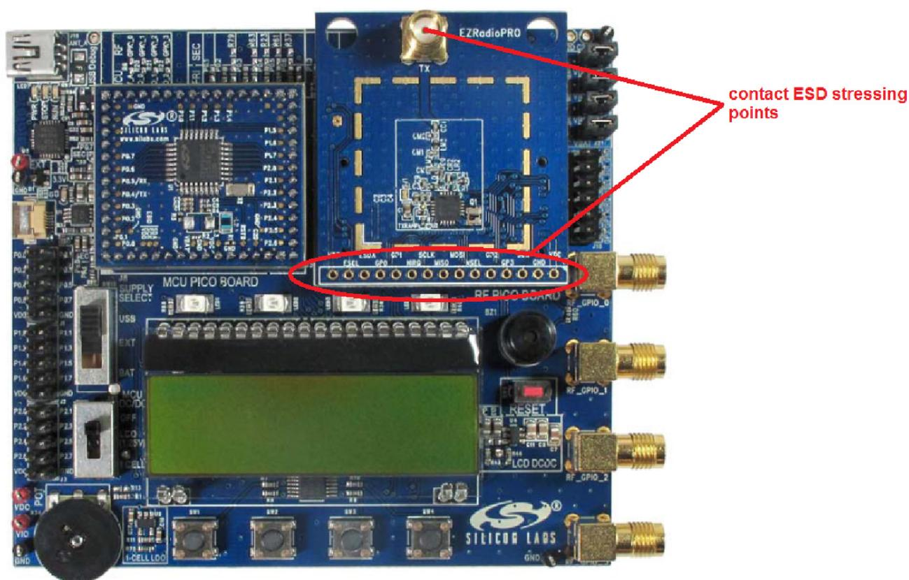
Figure 17. Wireless Motherboard with RF Pico Board Connected
