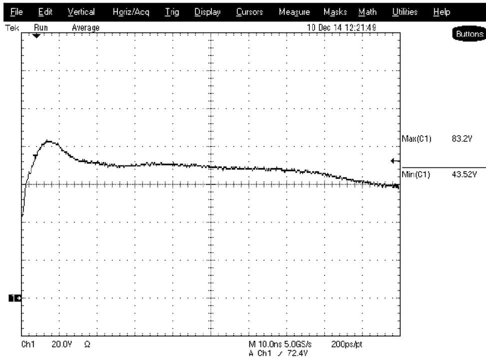
Figure 13. IEC 61000-4-2 Test Signal, +2 kV, 2 TVS Diodes and C1 = 2 nF, C2 = 33 pF, R = 15  $\Omega$  Mounted
