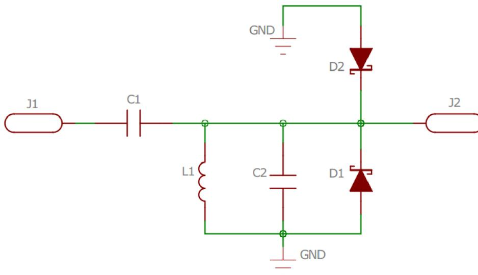
**Figure 19. ESD Protection Circuit for RF Antenna Port**
