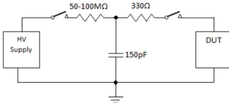
**Figure 2. Simulation Circuit of IEC 61000-4-2**
