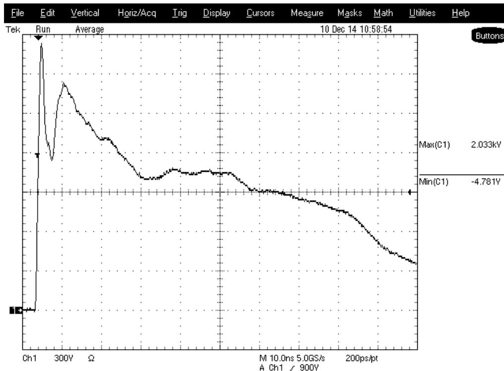
Figure 5. IEC 61000-4-2 Test Signal, +2 kV, without Protection
