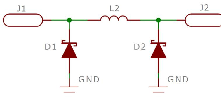
Figure 20. Additional ESD Protection Circuit in the RF Path
