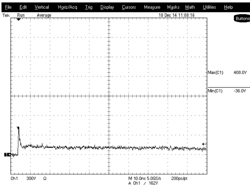
**Figure 7. IEC 61000-4-2 Test Signal, +2 kV, TVS Diode Mounted**
