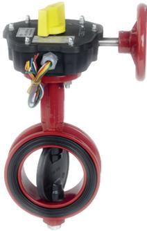
DCT28 Traceable Butterfly Valves are crucial components designed for controlling the flow of liquids and gases in a variety of industrial and commercial applications. These valves feature a robust, wafer-style body with a disc that pivots on a single axis, providing precise flow control. The wafer design facilitates easy installation between flanges and is ideal for applications where space is limited.
