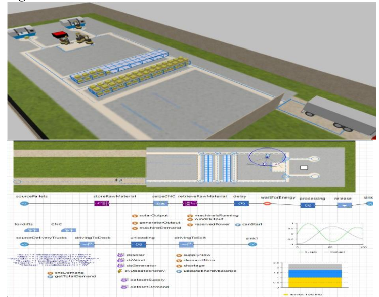
Figure 5: Running simulation in AnyLogic showing truck arrivals, CNC machine activity, and real-time energy metrics.
