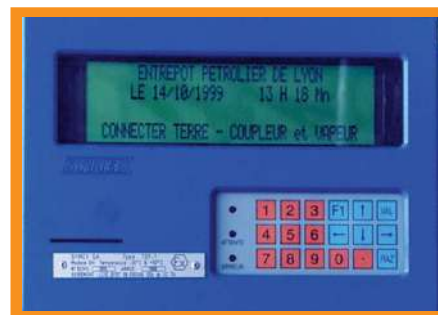
Identification terminal (badge reader), RFID technology
