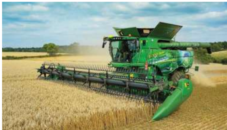
Figure 3: A combine harvester, used for harvesting, threshing, and cleaning grains.
