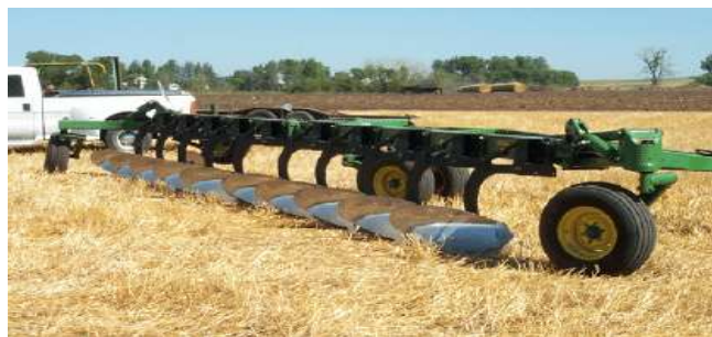
Figure 2: A moldboard plow, used for cutting and inverting the soil.
