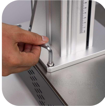
2. Fix the lifting column with four screws
