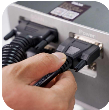
5. Insert the connecting line behind the laser
