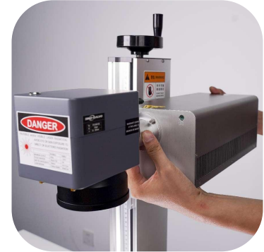
3. Place the laser on the column bracket
