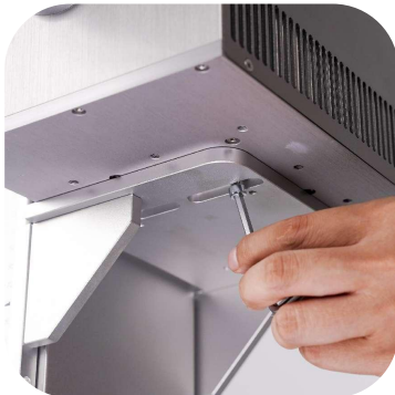
4. Four screws to fix the laser
