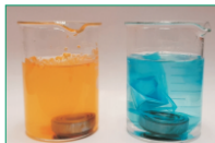
Vapro VBCI 826 SoluPlast totally dissolved in seawater
