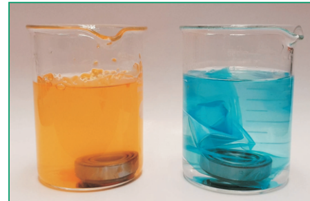
Vapro VBCI 826 SoluPlast totally dissolved in seawater
