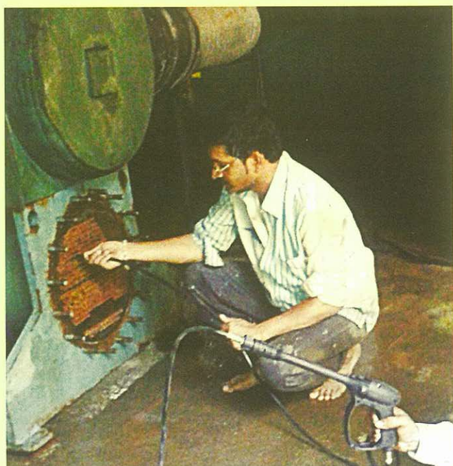
Figure 2: Mechanical tube brushing after chemical circulation
