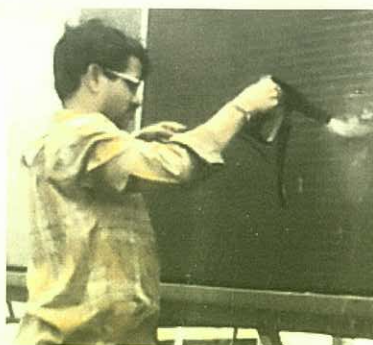
Figure 8: Mist spray of a small comfortable gun hitting an air cooled chiller coil at 90°
