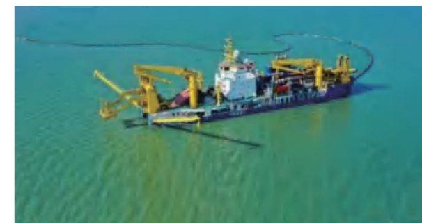
亚洲最大重型自航绞吸船“天鲲号” Asia's largest heavy self-propelled cutter suction vessel "Tiankun"
