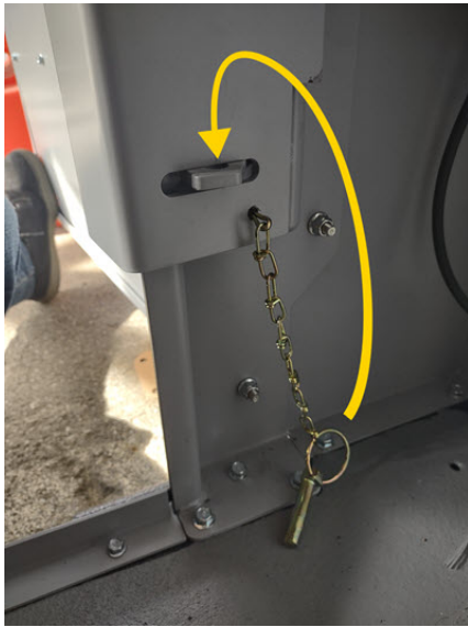
Locking tab and pin for the maintenance door.
