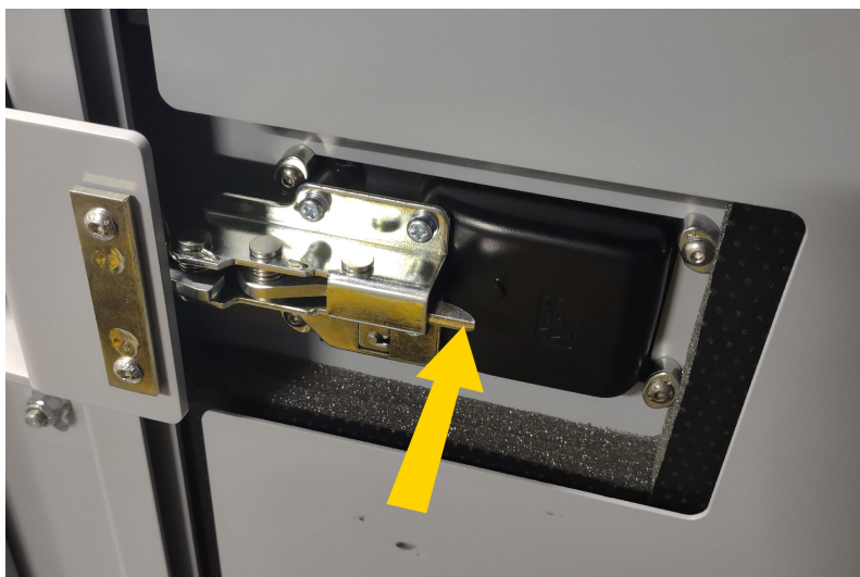
Egress latch on the inside of the maintenance door.
