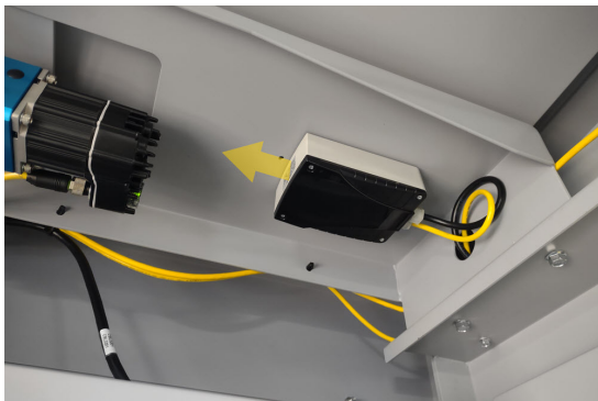
Detaching the RFID reader from the ceiling.
