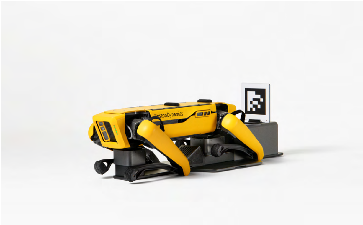
Charging a battery in Spot with the Spot Dock.
