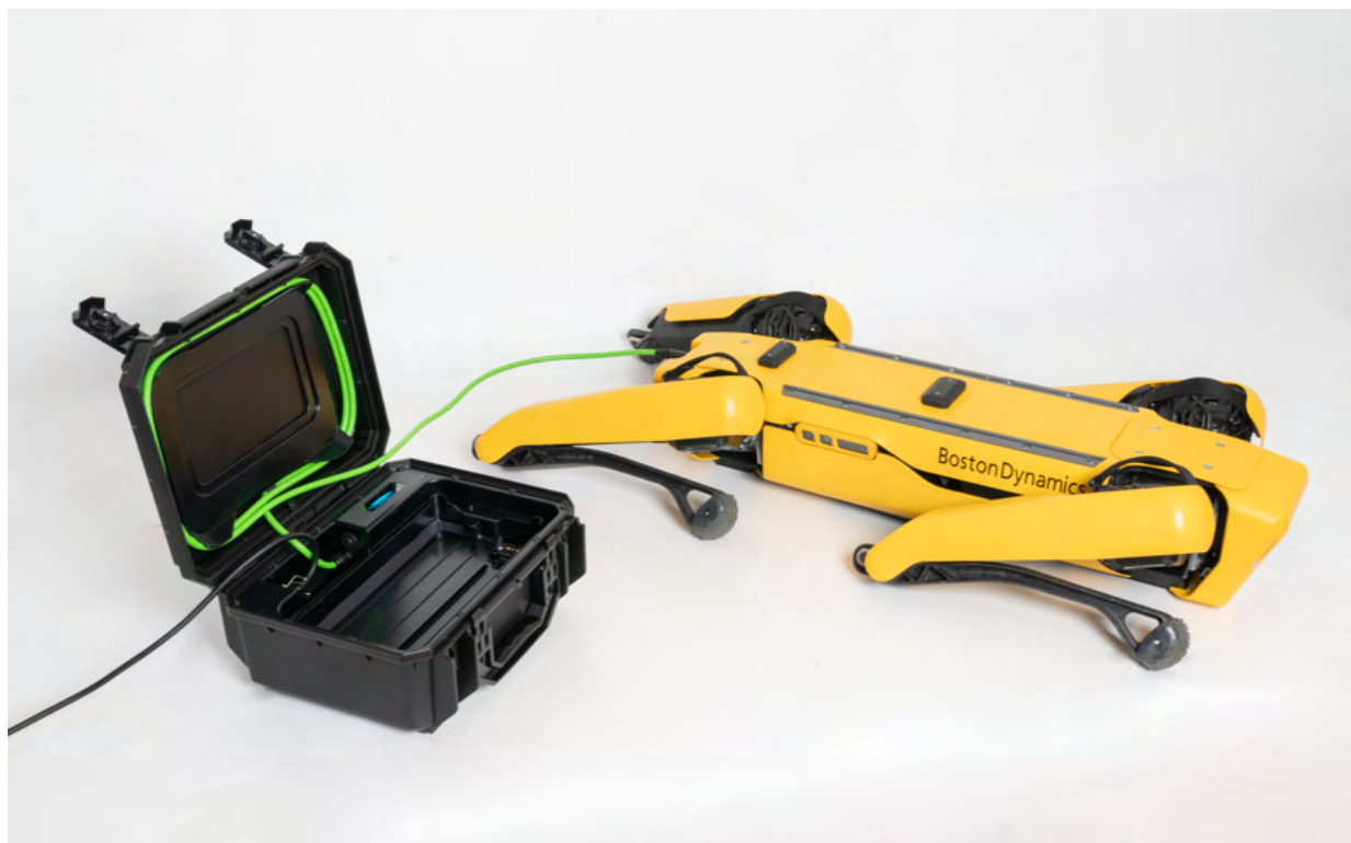
Charging a battery in Spot with the Spot Power Supply.
