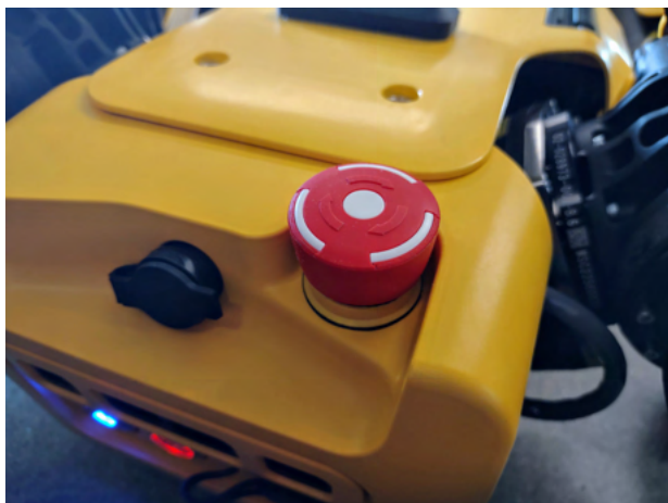
Spot's E-Stop button. Press firmly to activate; twist clockwise to release (unlatch).
