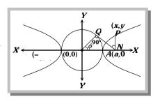
Here P and Q are the corresponding points on the hyperbola and the auxiliary circle  $(0 \le \phi < 2\pi)$
