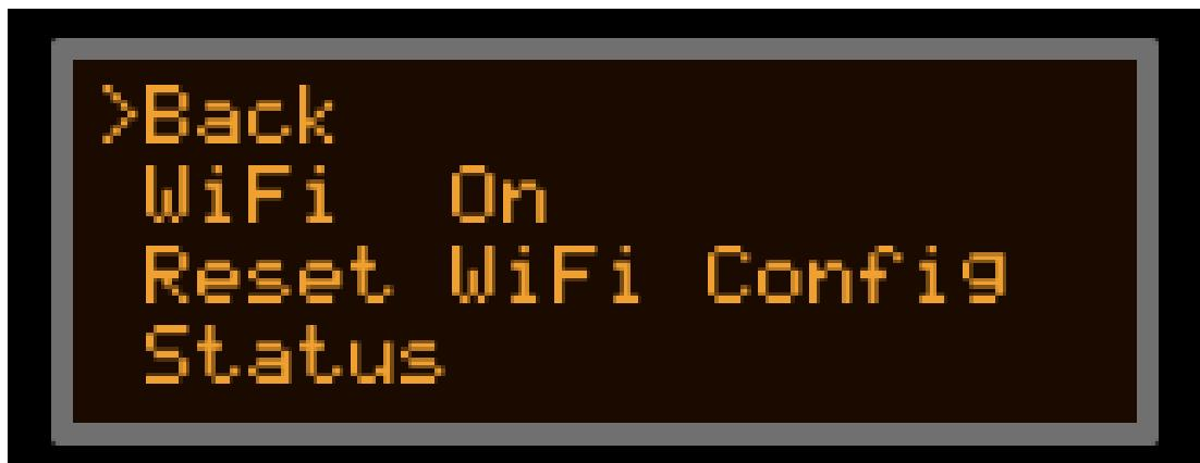
The Wi-Fi connectivity can be switched off if the user wants to save battery or it needs to avoid interference between other devices of the network. The user can switch it off by clicking the Wi-Fi tab and selecting 'Off'.
