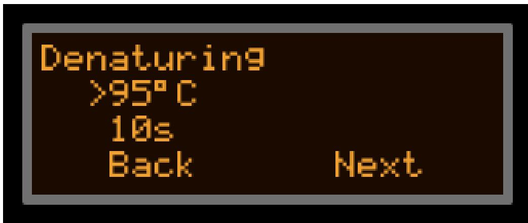
The second stage is Denaturing, the user should define the Temperature in Celsius, the duration in seconds. There is a choice to go 'Back' in the main menu or select 'Next' to continue with the definition of the bio protocol.
