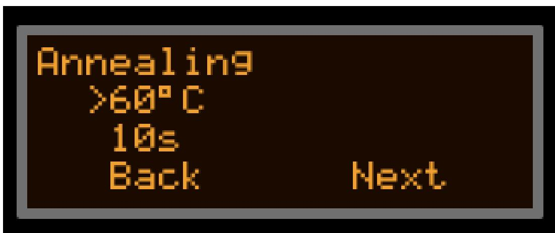
The third stage is Annealing, the user should define the Temperature in Celsius, the duration in seconds. There is a choice to go 'Back' in the main menu or select 'Next' to continue with the definition of the bio protocol.
