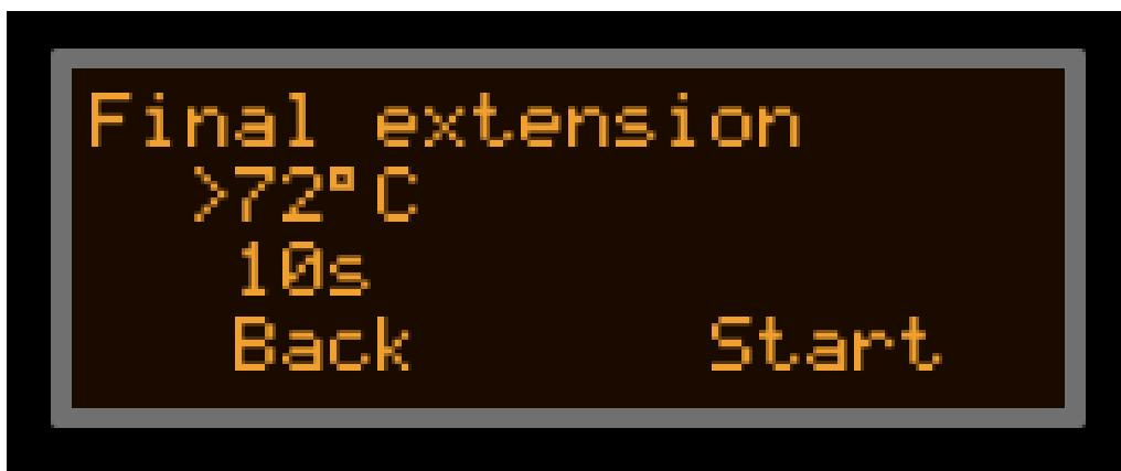
The fifth stage is Final Extension, the user should define the Temperature, the duration in seconds (min 10 seconds, max 5 minutes. There is a choice to go 'Back' in the main menu or select ' Start ' to finalize the definition of the bio protocol. After successfully defining all the stages then a message 'Bio Protocol defined' appears and the thermocycler will start to procedure all the commands.
