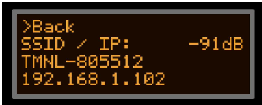
The network information the user can view the SSID of the router, the IP, the signal strength in dB, these information are important if the user forgets in which mode or network connected and it will be very useful to know.
