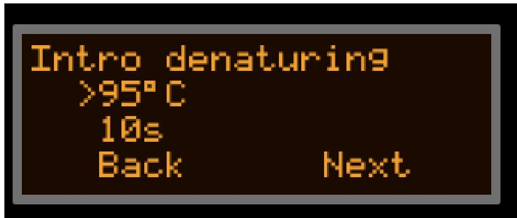
The first stage is Intro Denaturing, the user should define the Temperature, the duration in seconds (min 10 seconds, max 10 minutes. There is a choice to go 'Back' in the main menu or select 'Next' to continue with the definition of the bio protocol.
