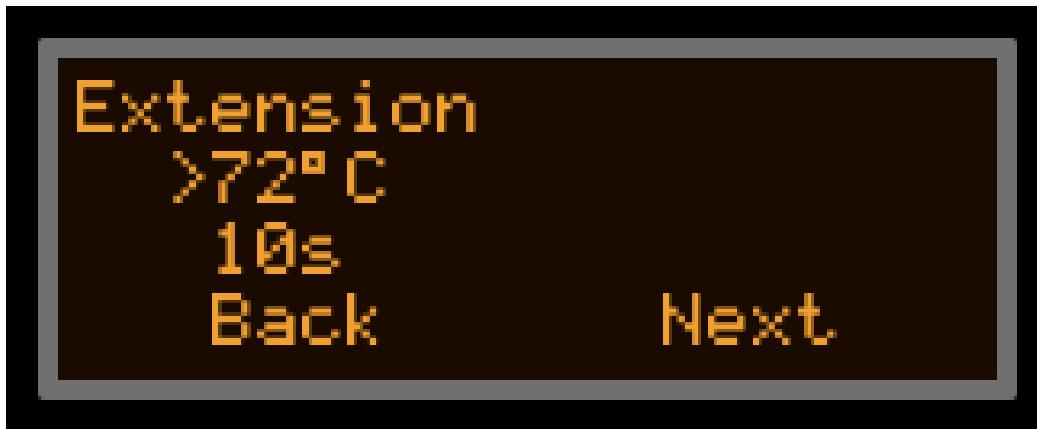
The fourth stage is Extension, the user should define the Temperature in Celsius, the duration in seconds. There is a choice to go 'Back' in the main menu or select 'Next' to continue with the definition of the bio protocol.
