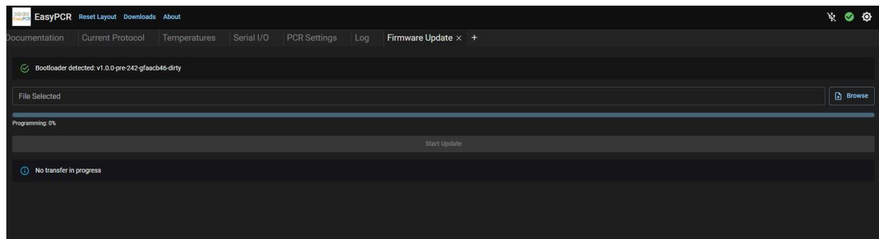
Please do not disconnect the USB-C cable , this process will take around 2 minutes. When the upgrade is successful the device will automatically reboot and you will see the intro message and the main page with the temperatures of the LID and peltier.
