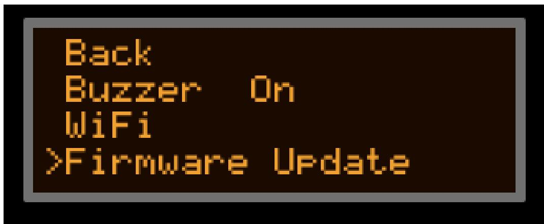
The user can update the firmware when there is a new version but the following steps need to follow. Connect a usb-c cable in the device, select in the LCD menu Firmware Update and in the menu are you sure click 'Yes'. Next step is to open a browser and type [ui.easypcr.io](http://ui.easypcr.io), select the bootloader USB connection. Last step select the firmware and click update, wait till complete the process 100%.
