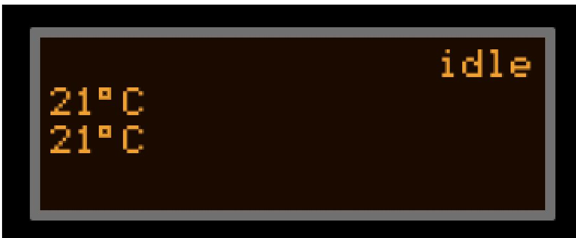
By clicking the push button a menu will appear in the LCD. Rotating the encoder the ' > ' will move and indicate in which sub-menu will select.
