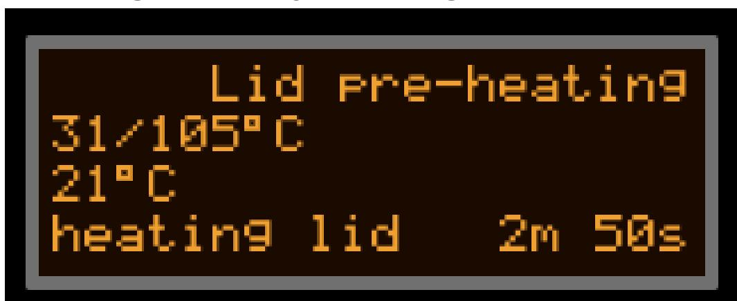
During the pre heating either of the LID heater or the hotplate block the red LED is active, while the BLUE led is active when the cooling part is applied in the bio protocol. During the bio protocol the user is able to abort the protocol by clicking the rotary encoder and click 'YES'
