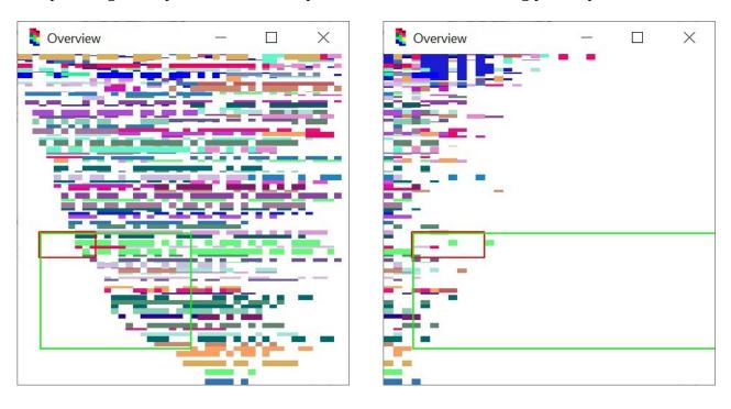
The presentation range in the **Arrangement** window is shown here with a red frame. The extent of the plan to be printed is shown here with a green frame.
