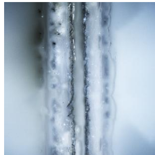
Fig. 2. Example of micromodifications (a side-hole along the length of the hollow-core fiber) made by a femtosecond laser beam.
