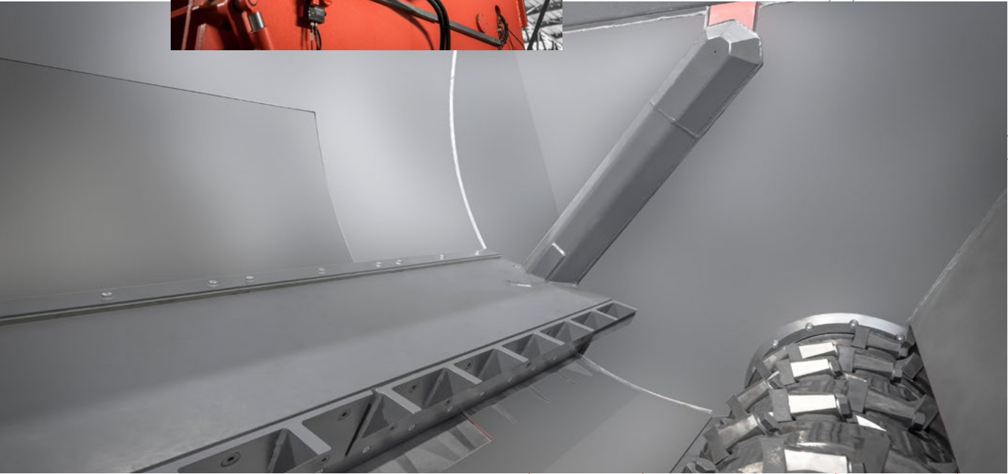
Hydraulic swing ram with robust lever and swingarm bearing
