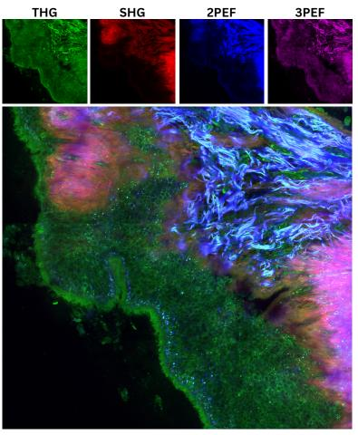
Higher harmonic generation (HHG) microscopy. The Flash Scanner FS4-R simultaneously acquires third harmonic generation (THG), second harmonic generation (SHG), two-photon (2PEF) and three-photon (3PEF) excited autofluorescence signals to provide complementary information about biological specimens. This image shows a bronchoscopy biopsy with cilia covered epithelium and stroma including elastin and collagen fibers.
