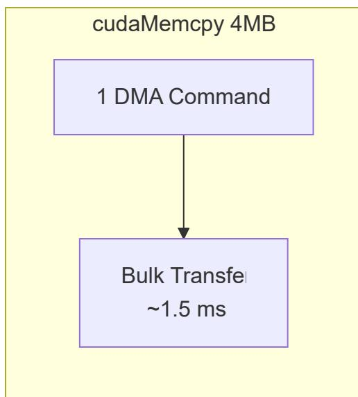
For large buffers, Unified Memory incurs page fault overhead: | Buffer Size | Pages (64 KB each) | Estimated Fault Overhead | |-----|-----|-----| | 256 KB | 4 | | ~200 us | | 1 MB | 16 | ~800 us | | 4 MB | 64 | ~3.2 ms | | 16 MB | 256 | ~12.8 ms | The DMA engine's bulk transfer capability becomes more efficient above 1 MB.
