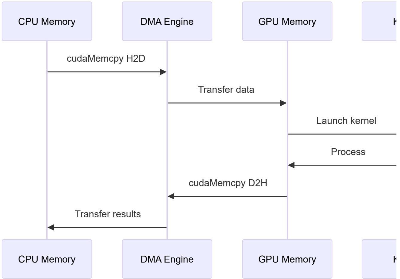
This pattern introduces significant latency overhead, especially for small buffers where transfer setup time dominates actual data movement.
