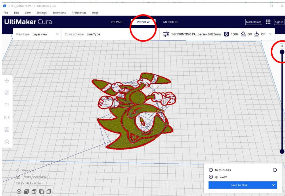
**Next is to add a code to stop every 2 layer to change the Syringe Cartridge with different Color.**
