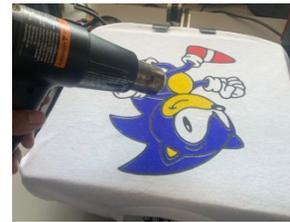
2. After complete printing you have to heat up the shirt Using heat gun, Heat presses or even iron to dry good .
