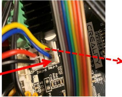
Laser engraver is connected on board **KF1 Fan**
