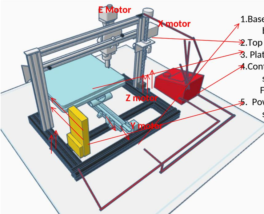
1. Base –connect to TOP – 2 screw for both side
