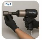
Fix the required socket and reaction arm on to the tool (fig.3).
