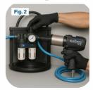
Set the required pressure as per chart provided, on the FRL while trigger pressed in torquing direction(fig.2).
