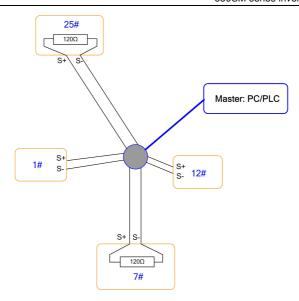
Notice: the furthest one (25#) and second furthest one (7#) inverters should connect the terminal resistor.
