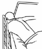
Zone 6 – Entrapment between the end of the rail and the side edge of the head or foot board
