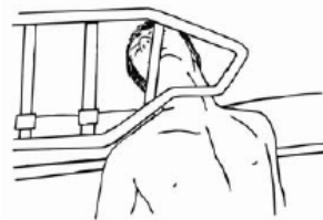
Zone 6 – Entrapment between the end of the rail and the side edge of the head or foot board
