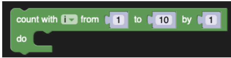
Fig. 35: The count block advances a variable from the first value to the second by the increment amount and running the do block once for each value. The block will count up with a positive increment and can count down with a negative increment. Typically 1 is used for the increment, but it can be any value, such as 2 to count even or odd numbers.
