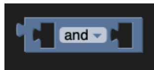
Fig. 28: Logical operators combined with relational operators let you create more complex boolean (true or false) expressions. The logical operators are OR (either of 2 operands are true) and AND (both operands are true). The result is true depending on the operands and the operator used.
