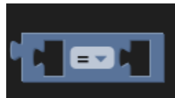
Fig. 27: Relational operators express the relation between values as true or false. There are 6 choices of relational operators, equals, not equals, greater than, less than, greater than or equals and less than or equals.
