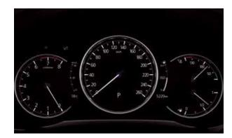
The three-meter cluster features a seven-inch TFT LCD colour display in the centre. In addition to vehicle speed, it shows diversified vehicle information in a clear, easy-to-read manner near the centre of the driver's line of sight.
