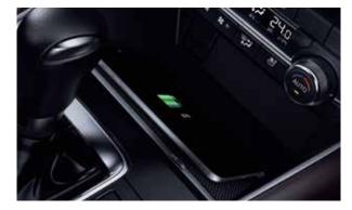
The centre console tray includes a Qi wireless charger\* to enable charging of compatible smartphones and other devices placed on it when the engine is running.
