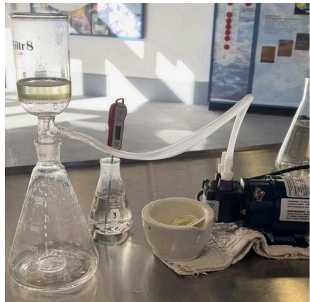
**Figure 5** Vacuum filtration setup
