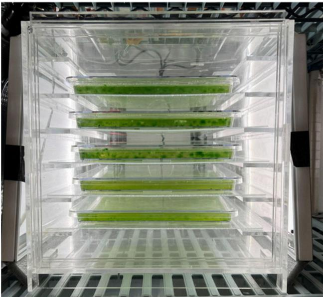
**Figure 3** Functioning photobioreactor core.
