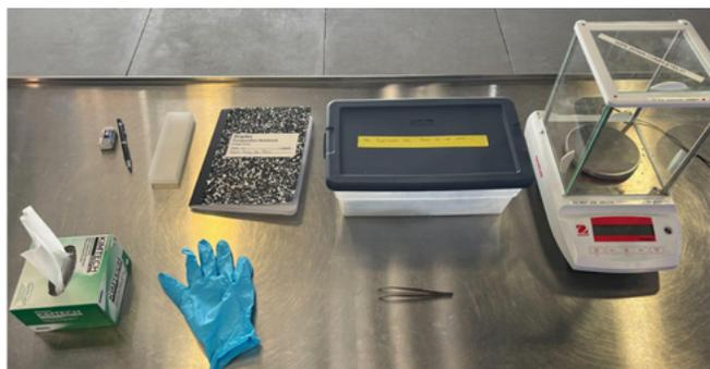
**Figure 7** Scale setup for biomass measurement
