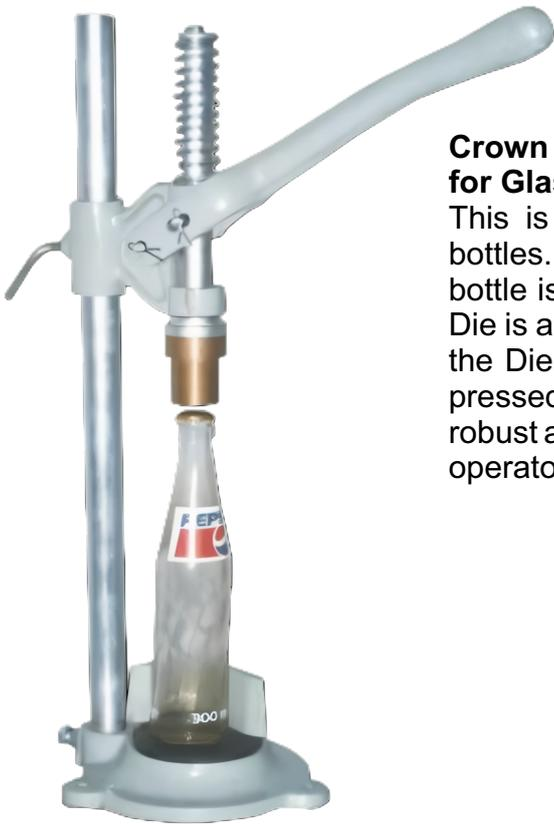
**Crown Capping Machine – Hand Operated Table Model – for Glass Bottles**
