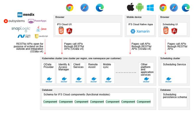
When deployed in the IFS Cloud Service (SaaS), IFS utilises Azure DevOps CI/CD pipelines with HELM charts for automating deployment tasks. Release deployments can be triggered by customers using self-service Application Lifecycle Experience Portal (ALE). A monitoring stack is also deployed for analysing various logs and metrics to keep the customer environments running smoothly.
