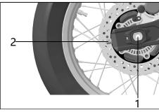
Fastening torque of adjusting nut: 22NM Fastening torque of rear wheel axle: 95NM
