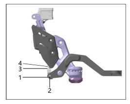
The free travel of rear brake pedal: 25-35mm
