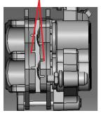
Limit abrasion position for rear brake pads:
