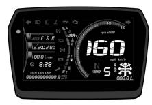
Tire pressure display: Match the sensor for tire pressure, show you the current pressure in Front/Rear tire. When the pressure is  $\leq 1.9$ bar or  $\geq 2.9$ bar, the mark of tire pressure and its corresponding "F" or "R" flashing and alarming.
