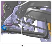
Driver with passenger and 3 cases, turn the adjustor 1 clockwise by 3 rounds.
