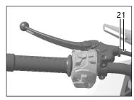
The free clearance at the end of clutch lever: 5-8mm.
