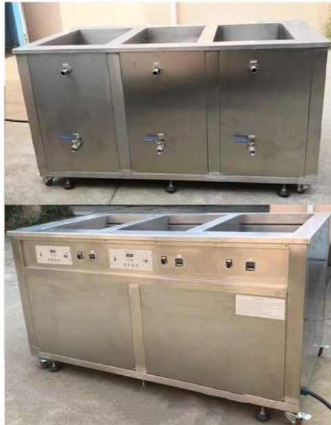
Ultrasonic washing device
