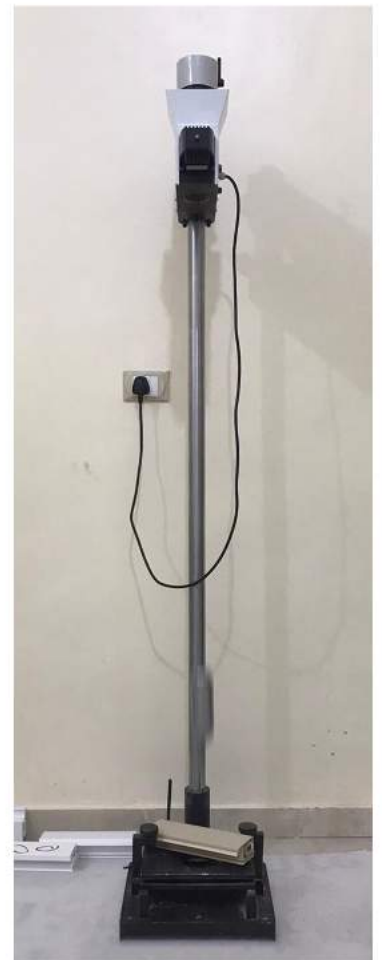
Falling impact device
