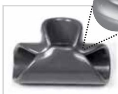
As the material flows together, a knit line starts to form.
